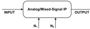
Figure 3.4: Block diagram of an analog/mixed-signal IP with two digital tuning knobs ( N_1, N_2 )
