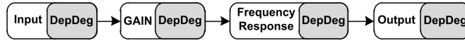
Figure 3.24: Block diagram of the behavioural model of an operational amplifier (OpAmp) with degradations
